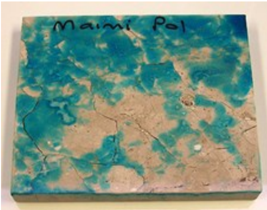
Figure 3. An example of a stone tile with significant potential for moisture marking.
