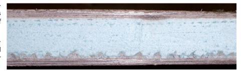
Polymer – cement combination with fibre-glass mesh reinforcement
