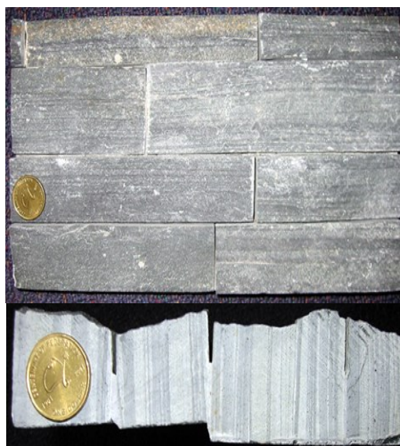
Figure 3. In case the stack is made from Quartz Mica Hornfels which has been epoxy glued parallel to the laminations. This rock is very hard and strong and does not easily fracture. When looked at carefully in hand specimen the quartz crystals can be seen glittering and the broken faces look 'sugary' in texture. As a tile, this type of rock is very durable, however the weight of this particular sample worked out to be 90\text{kg/m}^2 which is too high for adhesive only fixing and also too great for the substrate which de-bonded. Adhesive and mechanical fixing are required.
