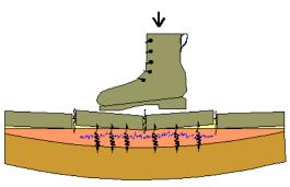
Where the deflection exceeds the recommended limits, or the maximum permissible movement for the adhesive, the adhesive can shear which will result in de-bonded tiles and cracked and popping grout.
