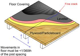
Excessive deflections in the floor can lead to cracking at the sheet joints. This won't effect carpets, but can lead to show-through for vinyl flooring.
