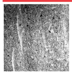
The attached photo is particleboard flooring sanded with 36 grit abrasive to produce a suitable textured profile clean of surface waxes and contaminants.
